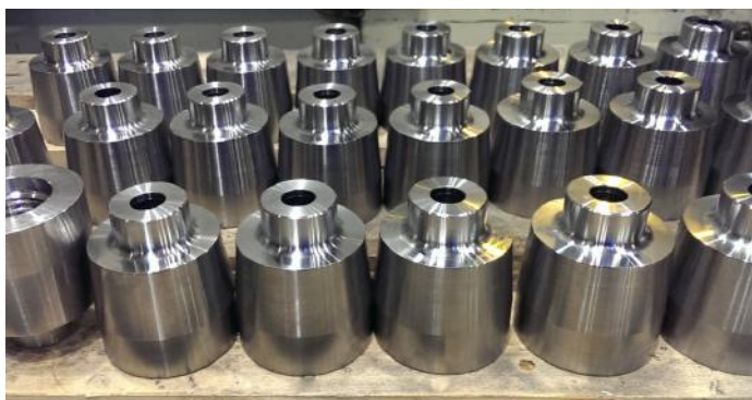
Slag Remover Attachments - Toolox 44 replaced W.Nr. 1.2344 to increase service life.
