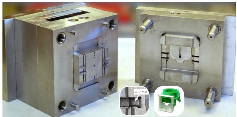
Top - Plastic mug produced with 15% lower cost than H13 / 1.2344 Bottom - PA6 electrical cover. Toolox 44 replaced AISI 420 to save production time.
