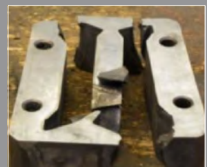
D2 / 1.2379 at 60 HRC crack after 10,000 shots
