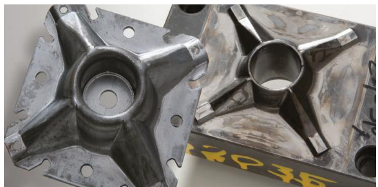
Top - Press tool with Toolox 44 for base plate in Electrolux refrigerator. Made 1,600,000 pieces. Bottom - Forming die. Toolox 44 produced 3x lifetime of D2 / 1.2379 (60 HRC)
