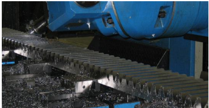
Gear Rack - Toolox 33 gas cut and machined. Much longer life than 42CrMo4.
