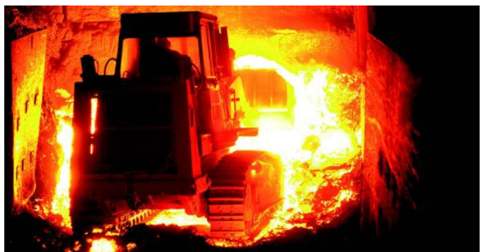
Hot Bucket - Toolox 33 had a lifetime of 8 months vs 8 weeks with other materials.
